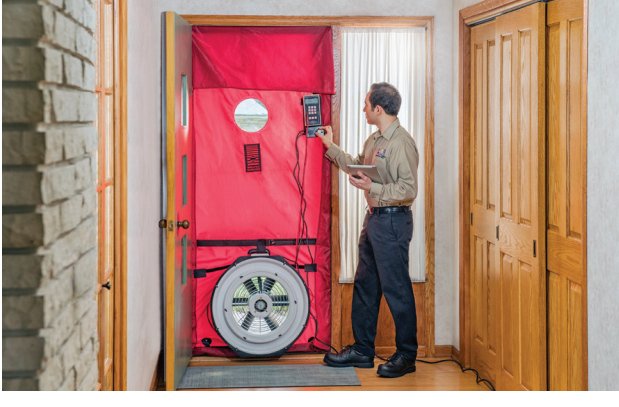
A HOME ENERGY SQUAD EXPERT performs a blower door test to identify potential air leaks in a home. (Submitted Photo).
